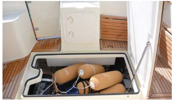
Tidy decks. Cockpit storage is provided by a usefully-sized lazarette compartment
